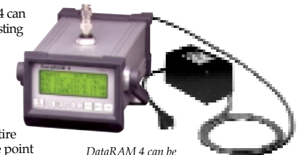
DataRAM 4 can be powered by a rechargeable internal battery or an external power source
